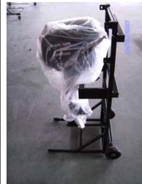
Unique hand cart that can be used also as metal fram shipping container
